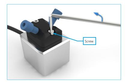
During reassembly, pay attention that the O-ring seal is placed correctly in the recess of the housing. Then put the housing back on and tighten the two screws evenly.
