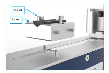
Mount the Contiflow valve using the supplied M3x8 Allen screws (2.5 mm Allen wrench) and washers as shown in the picture below.
