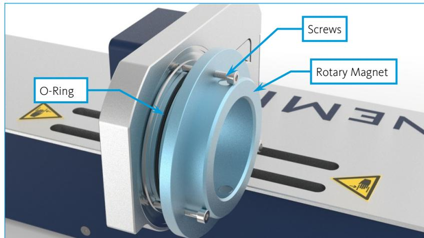
To make assembly easier, lightly lubricate the O-ring with some silicone grease and insert the magnetic ring. Push the drive wheel to the side and, to avoid tilting, press the magnetic ring straight and as far as possible.
