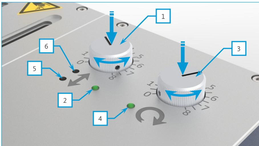
1. Pressing the adjustment knob **1** will toggle the lateral movement of the mixing assembly  $\updownarrow$ . When switched on, the green status LED **2** will be illuminated.
