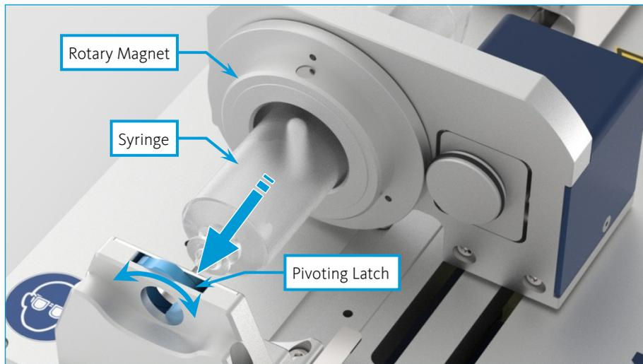
2. Then insert the syringe piston into the piston holder as shown in the following picture.
