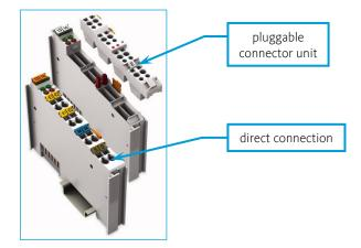
In both cases the cables are fixated by a spring-type terminal, that allows the use of solid, and stranded conductors.
