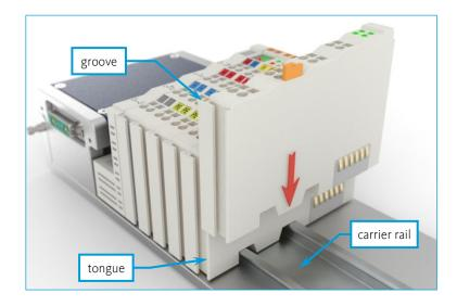
With the clamp module snapped in place, the electrical connections for the data contacts and power contacts to the previous or possibly subsequent clamp modules are established.
