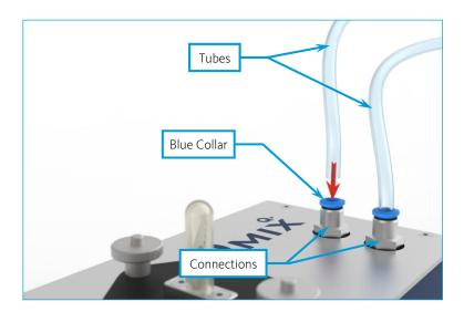
For example, tap water or ice water can be used as cooling liquid. Other liquids are also possible if they are compatible with NBR seals.
