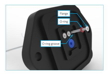
(4) Compress the rubber cap on the top side of the chip holder and insert the chip so that the connection openings of the chip and the flanged tubes align. Press the chip down on the suction cup and then release the rubber cap. The chip is now fixed and you can mount the chip holder onto the Qmix Q- module.
