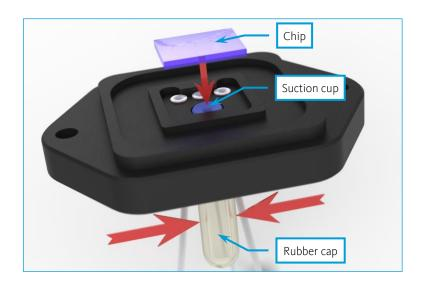
(5) Mount the chip holder on the Qmix Q- module. For this, remove the two knurled nuts from the locating bolts. Then slide on the chip holder onto the bolts and reassemble the knurled nuts. Tighten the nuts alternating and equally until they are finger-tight.
