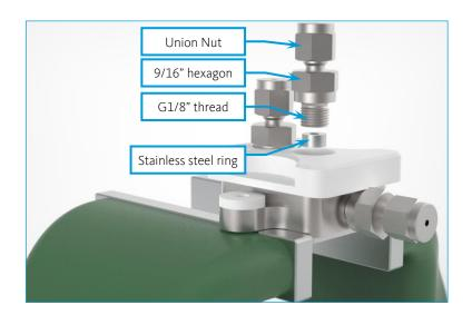
Depending on the type of tube fitting, capillaries with an external diameter of 1/16" or 1/18" can be used. For the Assembly or Disassembly of the tube fittings of the 1/16" version, you need a 5/16" openend wrench and for the 1/8" version you need a 7/16" openend wrench.
