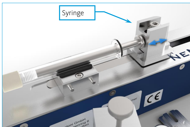
Fixing the Syringe in the Piston Holder
