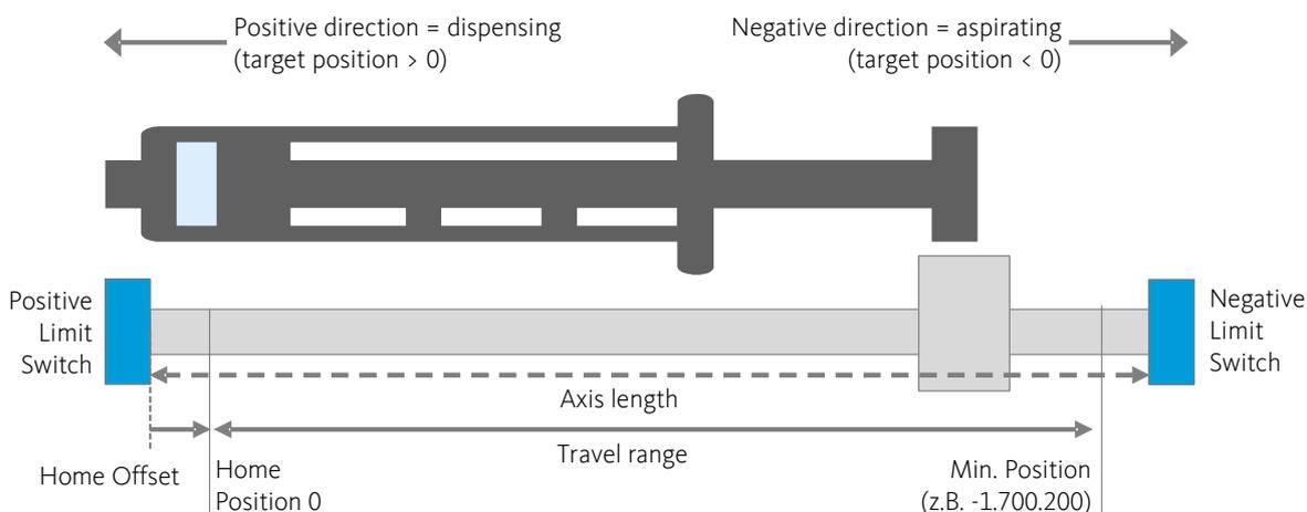
The physical *axis length* is the distance between the positive and negative limit switch. During normal dosing operations, the pusher should not reach the limit switches. Therefore the real *travel range* is limited by two offsets: the *Home Offset* on the *Positive Limit Switch* side and a second offset on the *Negative Limit Switch* side.
