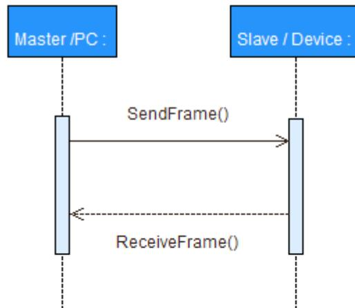
Figure 12: RS232 Communication – Command Sequence
