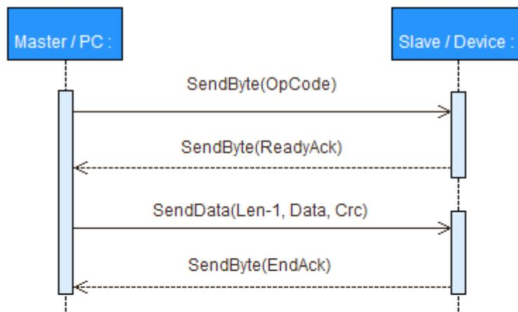
Figure 13: RS232 Communication – Sending a Data Frame to device
