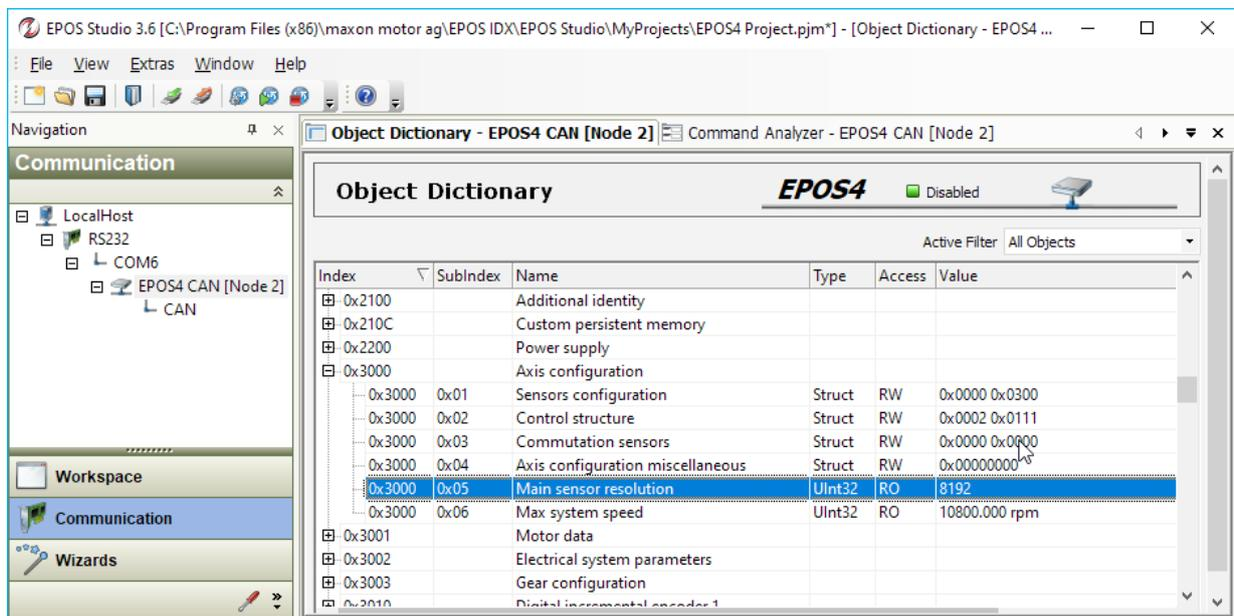
The EPOS Studio Command Analyzer will help you to analyze the low level RS232 protocol including checksum calculation. With this tool you can execute certain commands and access the object dictionary and you will see the corresponding serial protocol frames including CRC and stuff bytes.
