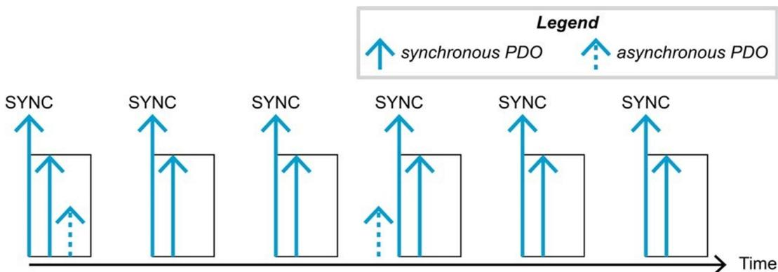
Figure 8: Synchronous PDO
