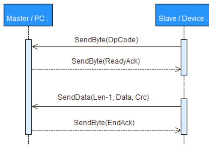
Figure 14: RS232 Communication – Receiving a response data frame from device
