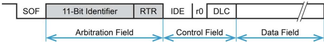
Figure 2: Standard frame format
